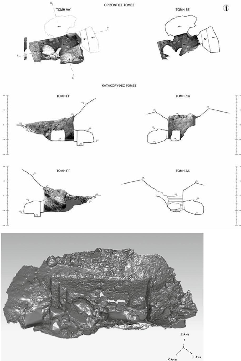
**Figure 10.38a–b:** The geometric documentation of grave 2/2006 on the Eastern Necropolis of Kymissala-Orthophotos (a) and 3D model (b) (KARP-NTUA).
